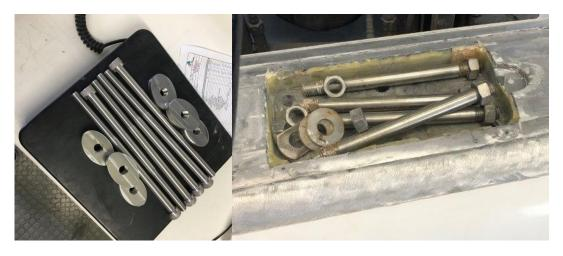
A.8.1.2 Under-fin spacer plates that fit between the keel fin & bulb
