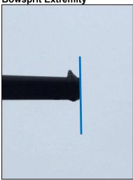
It is important to note that the measurement is taken to the extremity of the **spinnaker pole**, **whisker pole** or **bowsprit** and not to the bearing point of a spinnaker pole or the block/ferrules which the tack line passes through on a bowsprit.
