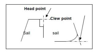
The batten shall be a standard 1m World Sailing blue batten unless the measurer cannot achieve a consistent measurement in which case the measurer shall use a batten of consistent bend characteristics and length appropriate to the sail being measured. The measurer shall provide photographs to the Rating Authority.
