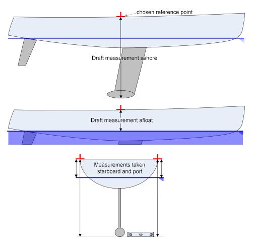
Draft = Draft measurement ashore – Draft measurement afloat
