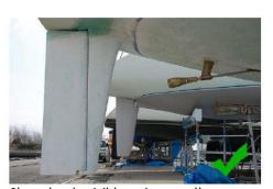
Skeg clearly visible as is propeller
